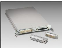
The Model 7707 plug-in module offers 10 channels of 2-pole or 5 channels of 4-pole multiplexer switching that can be configured as two independent banks of multiplexers. The Model 7707 also provides 32 digital input/output channels (four 8bit ports) for I/O control. Connect the Model 7707 to industry standard solid-state relays to switch up
